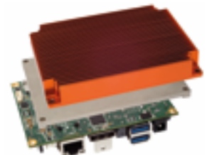
Cooler and heatspreader installed to bottom side of a Pico-ITX
