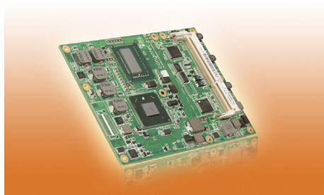
conga-TS77 COM.0R2.0 Type 6 module based on the third generation of Intel Core i7 processors
