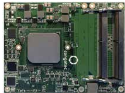
congatec's new COM Express Type 7-compliant server-on-module comes with Intel® Xeon® processors (codename: Broadwell DE).
