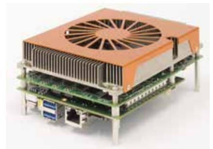
Measuring 125mm x 95mm, edge/fog server designs with Server-on-Modules have an extremely compact footprint.
