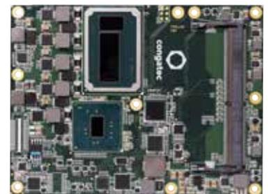
congatec COM Express Basic modules with Intel® Xeon® processors provide server-class computing performance and up to 32GB ECC DDR4 RAM.
