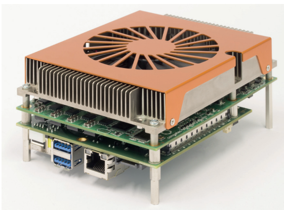
Figure 1: High-end performance compacted down into 125 x 95 mm: congatec TR3 computer module with active heatpipe solution mounted on a carrier board without loss of performance.
