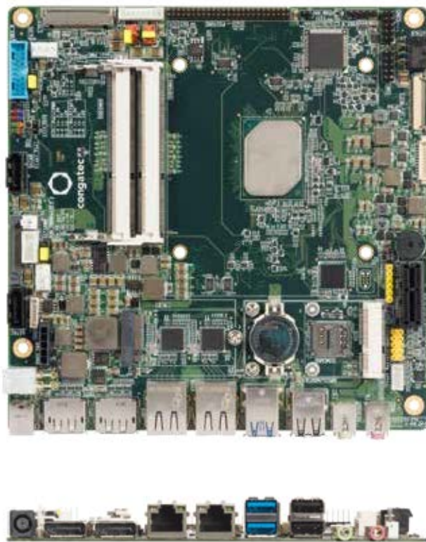
Thin-Mini ITX 170 x 170 mm 2 at a maximum height of 20 mm
