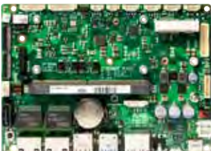
conga-SMC1/SMARC-x86 Carrier Board for x86 based SMARC 2.0 modules.
