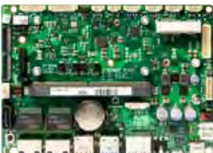
conga-SMC1/SMARC-ARM Carrier Board for ARM based SMARC 2.0 modules.
