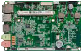
conga-MCB/Qseven Small size (95x140mm) carrier board to support all x86 based Qseven modules.
