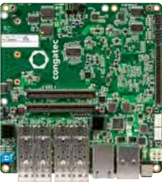
conga-STX7/Carrier Evaluation mini-STX carrier board for COM Express Type 7 modules.
