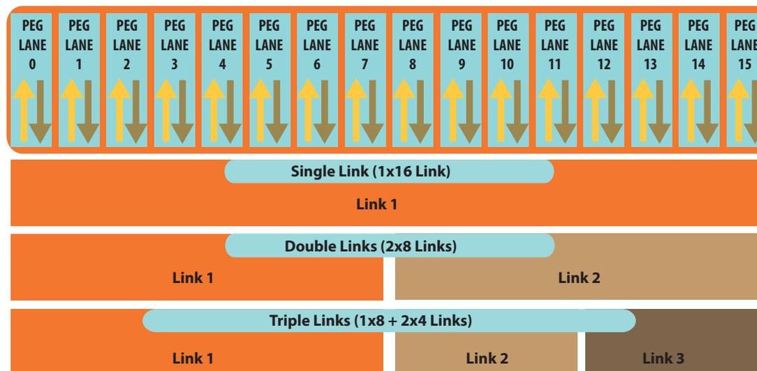
The 16 PEG lanes can operate at 2.5 GT/s, 5 GT/s or 8 GT/s. The PCIe lanes of the PEG interface are controlled by three controllers. Each controller can automatically operate on a lower link width allowing up to three simultaneous operating devices on the PEG interface. The PEG root port configuration can be selected in the BIOS setup.
