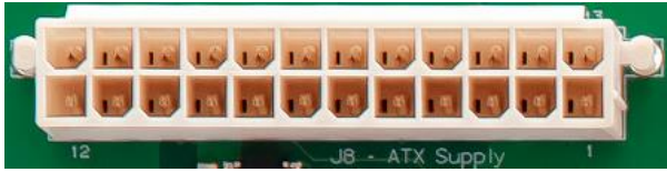
Figure 21: 6.16. 24-pin ATX Power connector (J8)
