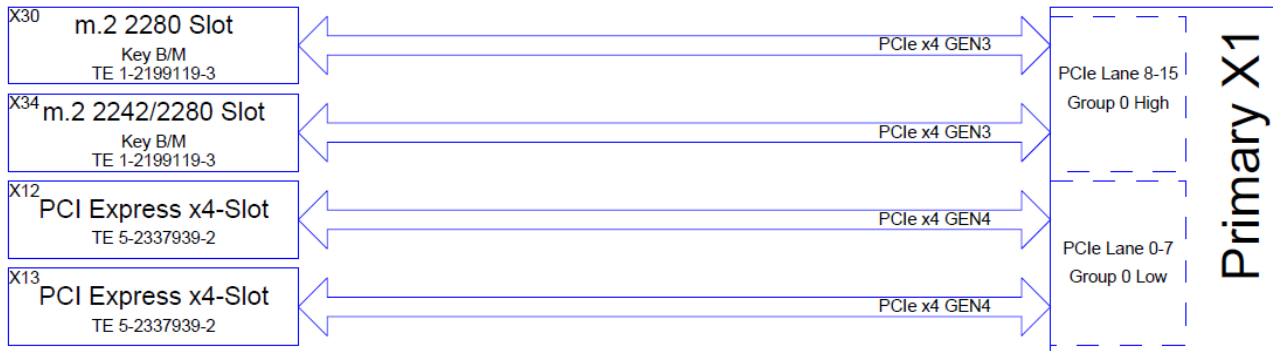
Figure 11: PCIe x4 Slots
