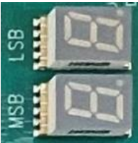
Figure 42: Port 80 BIOS Debug Code 7-Segment Display
