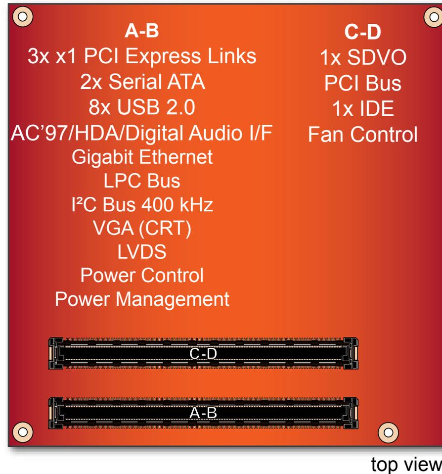
In this view the connectors are seen “through” the module.
