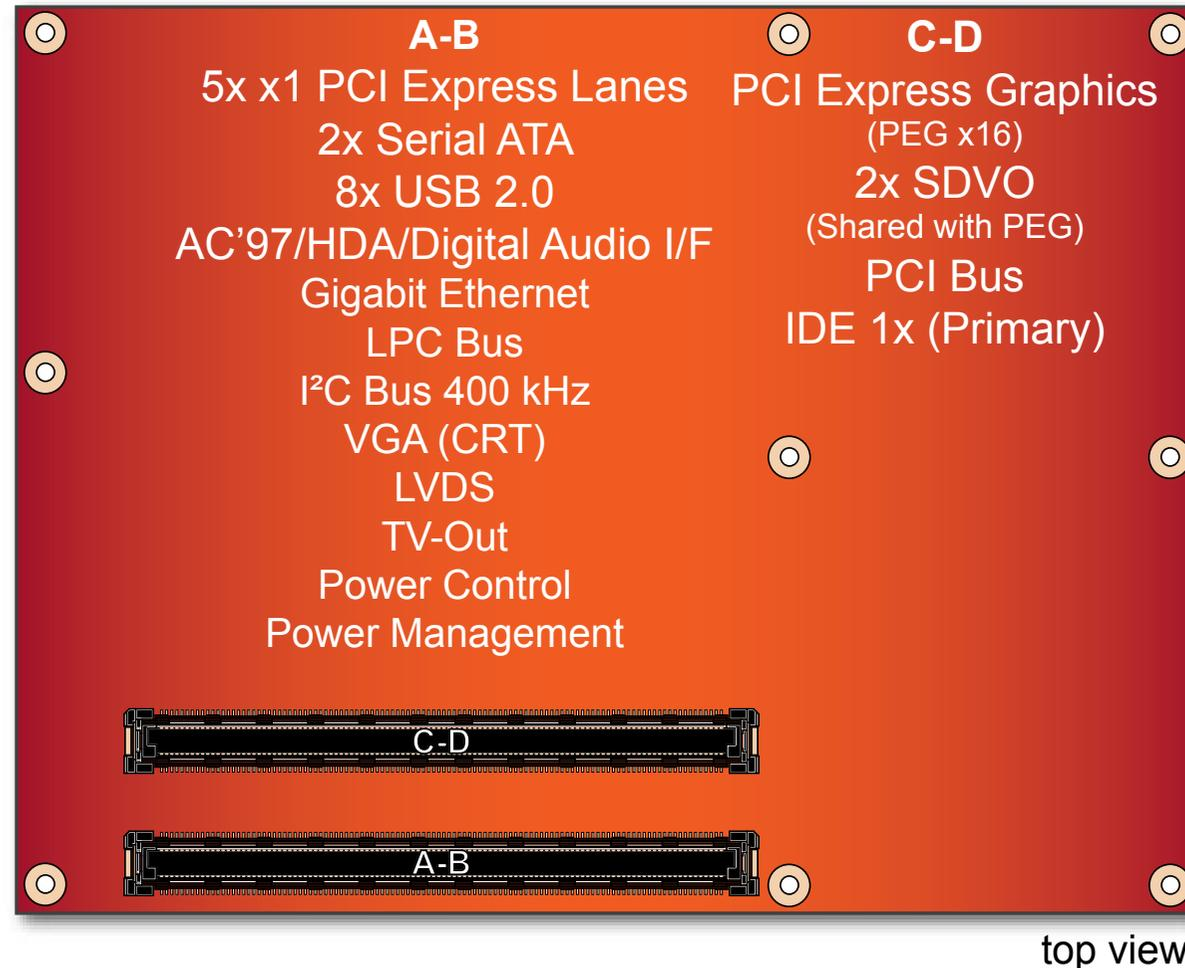
In this view the connectors are seen “through” the module.
