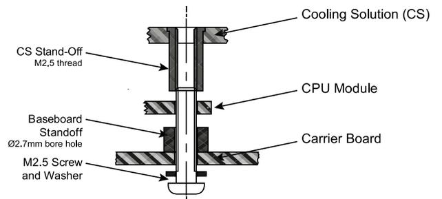
Bottom mounting scenario uses the threaded version cooling solution and requires bore hole standoffs on the carrier board.
