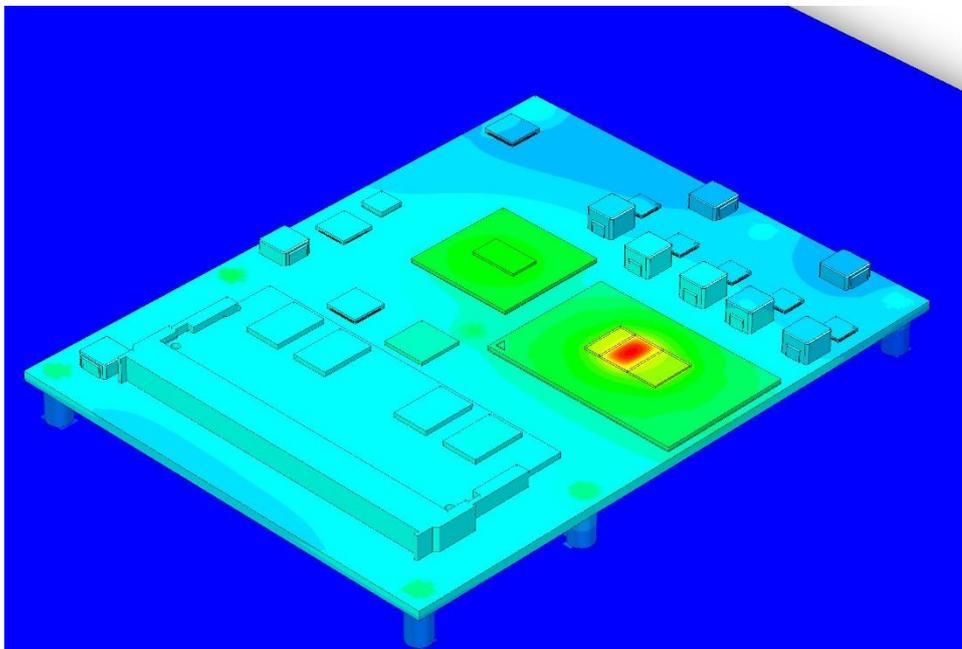
This shows the same simulation with a module only view to visualize the thermal state of the CPU and PCH. The hot spot is the CPU die, which does not exceed the allowed maximum temperature.
