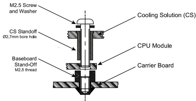
Top mounting scenario uses the bore hole version cooling solution and requires threaded standoffs on the carrier board.
