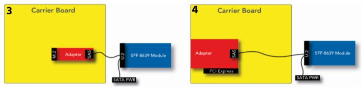
Topologies 3 and 4 use the HD Mini-SAS to U.2 cable as described in the first topology. Both setups can be used to determine the function of your U.2 module in existing carriers by using adapters on existing interfaces.
