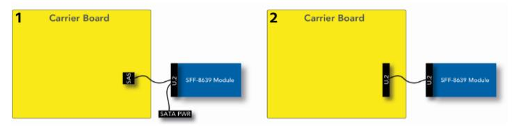
Cabling sets on the market right now focus on reusing existing SFF-8643 cables and connectors. These Mini-SAS HD cables are capable of carrying PCIe signals necessary for operating U.2 NVMe modules. Topology 1 depicts this setup. The carrier board features the SFF-8643 connector. An SFF-8643 to U.2 cable is used to connect the device. In addition, power is supplied to the U.2 module via a SATA power connector.
