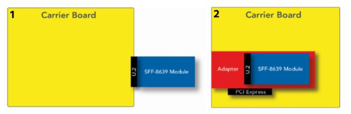
Topology 1 (left) connects a U.2 module directly to the standard connector. In this topology, SATA, SAS and U.2 NVMe modules can be connected if the carrier board connector supports all U.2 interfaces.
