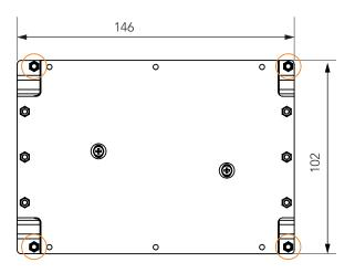
M2.5 x 8 mm threaded standoff for threaded version or ø2.7 x 8 mm non-threaded standoff for borehole version
