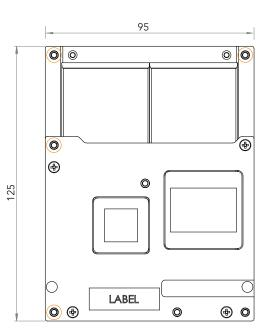
M2.5x11mm threaded standoff for threaded version or 2.7x11mm non-thread standoff for bore hole version
