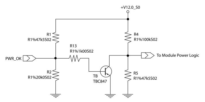
The voltage divider ensures that the input complies with 3.3V CMOS characteristic and also allows for carrier board designs that are not driving PWR\_OK. Although the PWR\_OK input is not mandatory for the onboard power-up sequencing, it is strongly recommended that the carrier board hardware drives the signal low until it is safe to let the module boot-up.
