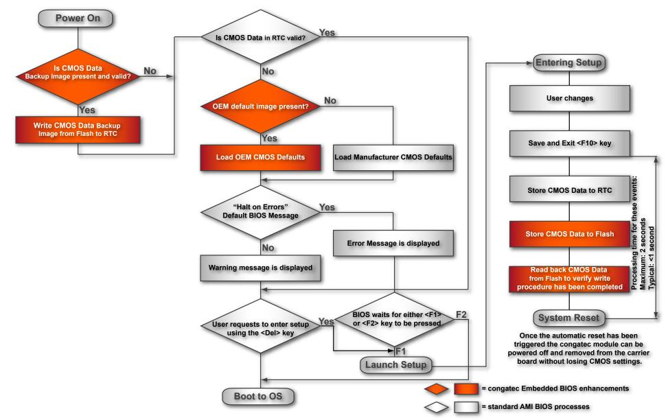
The above diagram provides an overview of how the BIOS Setup Data is backed up on congatec modules. OEM default values mentioned above refer to customer specific CMOS settings created using the congatec System Utility tool.
