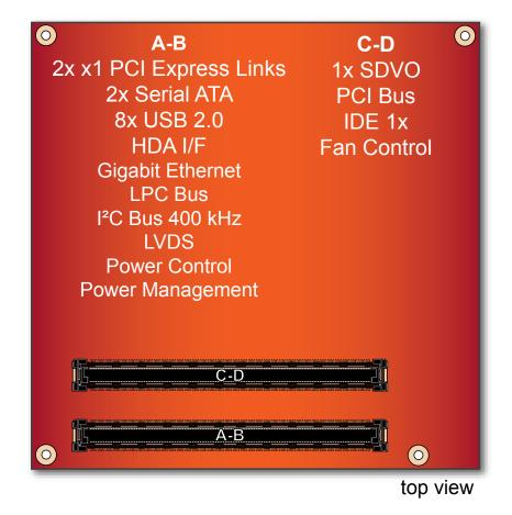
In this view the connectors are seen "through" the module.
