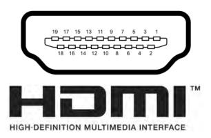
HDMI is supplied by the SDVO interface that originates from the COM Express™ Compact module as SDVO port B over DVI/HDMI Transmitter.
