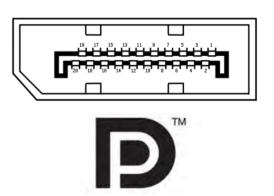
DisplayPort originates from connector XCD1 on the COM Express™ Compact module as DDI port C.
