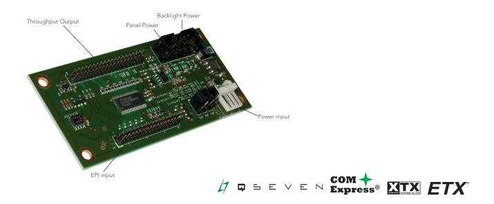
conga-FPA2 is a universal flat panel adapter board that has been designed to be EPI (Embedded Panel Interface) compliant. It can be used for either prototyping, demonstration purposes, or for debugging certain issues. It may also serve as a reference for the implementation of panel adaptations on customer specific carrier boards.
